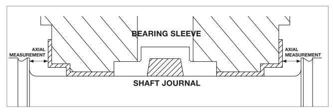
Figure 10-3: Bearing Mechanical Center
