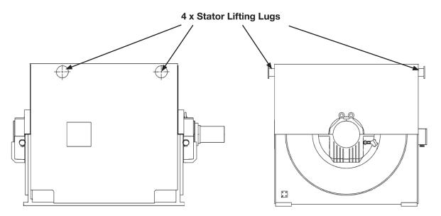
Figure 6-1: Handling of the Motor
