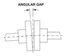
Figure 10-1: Parallel and Angular Misalignment Measurements
