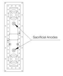
Figure 9-1: Radiator with Sacrificial Anodes
