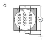
Figure 7-2: Connection of the Megohmmeter to Separate Phases
