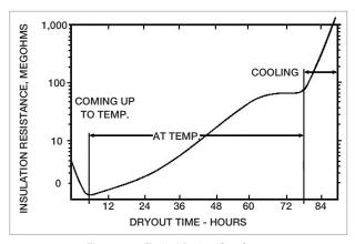
Figure 7-4: Typical Drying Out Curve
