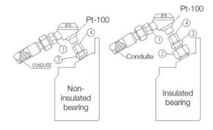
Figure 17-9: Pt100 on the Bearings
