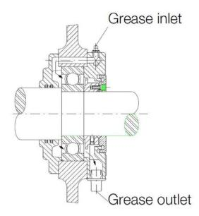
Figure 17-10: Grease-Filled Rolling Element Bearings
