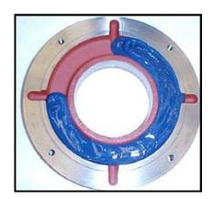
Figure 17-8: External Bearing Cap
